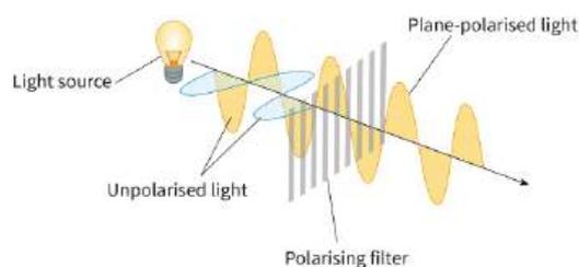
Figure 9. Plane-polarised light is produced by passing unpolarised light through a polarising filter.
